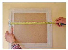
**2**. Measure across the frame the distance between the centres of the holes in the Bridge brackets. This may be done by measuring from the outside of one Bridge to the inside of the other as shown left.
